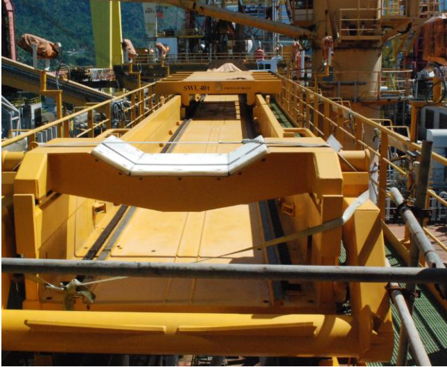
Pipe Catwalk DRU URCA
