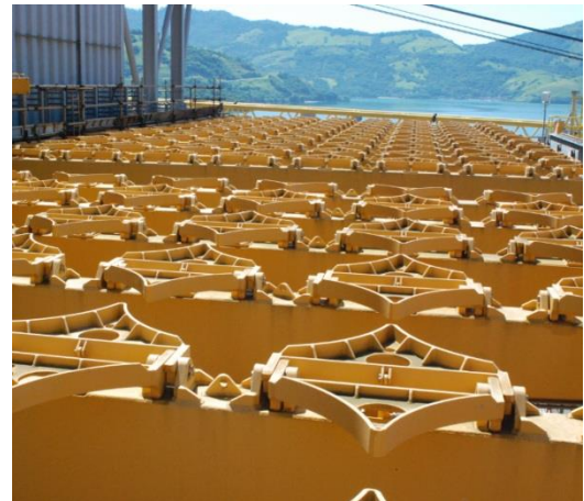
Riser storage area DRU URCA
